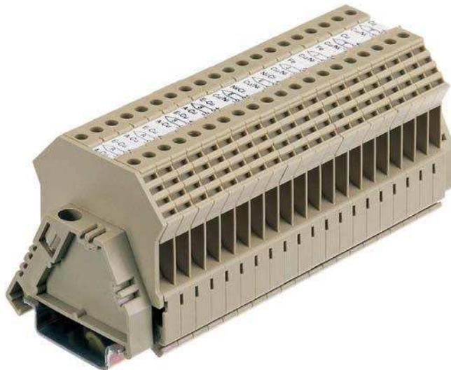
The **CONTA-CLIP TSK** terminals can be used to clearly label the thermal terminal pair in use. The busbars on the thermocouple terminals are made of the same materials as the compensating lines, in compliance with DIN 43713/DIN 43714. This ensures thermocouple signals are transmitted accurately on the junction between the thermocouple, thermocouple terminal and compensating line.
